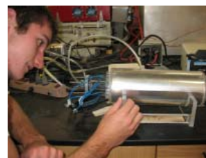
Photocatalytic reactor used to purify polluted water.
