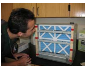
Filtration system impregnated with titanium dioxide for indoor air detoxification.
