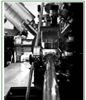
The thermo-chemical fuel project uses an ultra-high vacuum analytical tool which identifies the chemical species on the catalyst.
