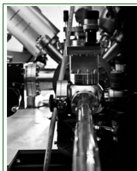
The thermo-chemical fuel project uses an ultra-high vacuum analytical tool which identifies the chemical species on the catalyst.
