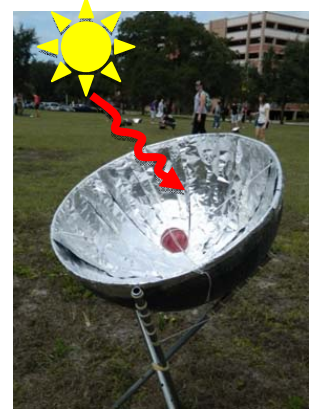
The winning concentrating solar oven from the team of Alexander Dalzell, Brandon Demers, Zahi Salloum, Dion Motl, and William Harrison.
