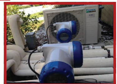
Refrigerant flow meters wired and connected to data logger system.
