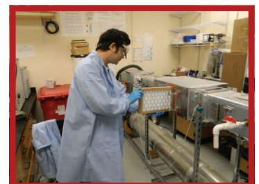
A titanium dioxide (TiO 2 ) infused filter is inserted into an experimental closed loop air duct.
