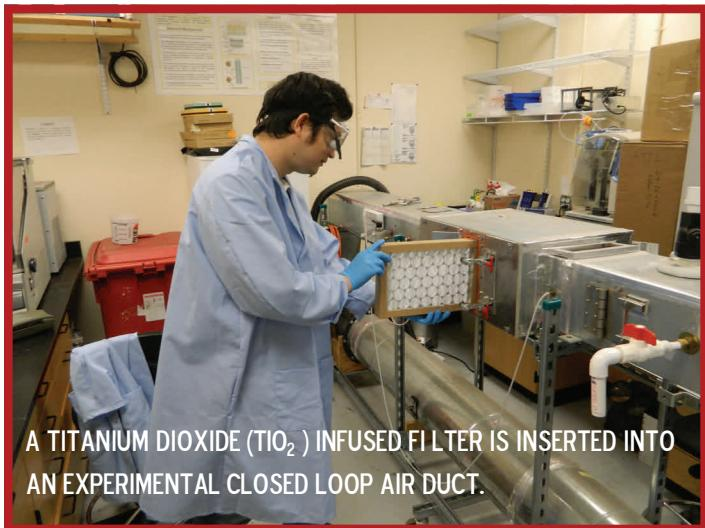
A TITANIUM DIOXIDE ( $TiO_2$ ) INFUSED FILTER IS INSERTED INTO AN EXPERIMENTAL CLOSED LOOP AIR DUCT.
